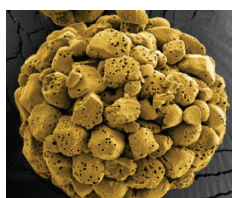
SEM (scanning electron microscope) image illustrates the morphology of N-ZORBIT™ 2144/2144 DG plating agent's agglomerated microporous starch granules.
